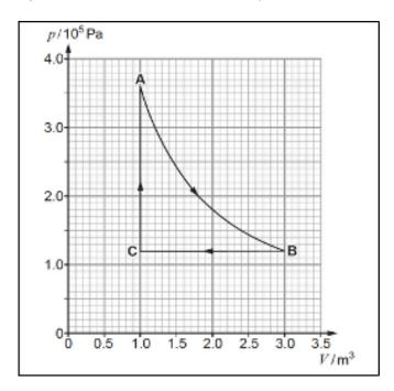
(i) Ian claims A  $\rightarrow$  B is an isothermal process. State what is an isothermal process and show this is an isothermal process.
