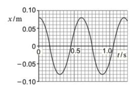
(i) Sally measured the equilibrium extension of the spring, when loaded with the 0.200 kg mass, recording it as 90 mm. Evaluate whether or not this is consistent with the period of the oscillations.
