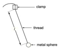
Using a metre ruler she measured the length, l, shown in the diagram. She then recorded the time for 10 small amplitude oscillations, repeated the timing and calculated values for the mean periodic time, T, and its uncertainty. She repeated the procedure for another five values of l. She plotted her values of  $T^2$  against l on the following grid.
