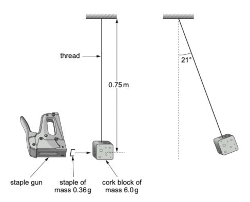
The cork block is set moving to the right by the collision, coming to rest momentarily when the thread is at an angle of 21° to the vertical.
